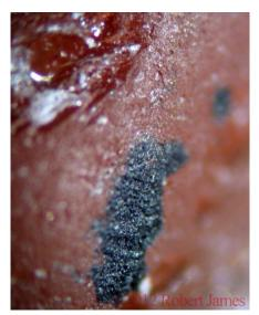
By Raman scan we found that this material you see at left is....graphite. And not just any graphite, this material is *annealed graphite*.
