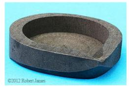
At left you see a graphite crucible that we obtained from a supplier who provided documentation that this crucible had been annealed to 1000°C. We were able to use this crucible as our control piece for our Raman testing and evaluation for annealed graphite.
