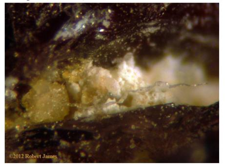
By Raman we have confirmed that this sodium silicate liquid that has so many uses may well be the culprit somehow in this unusual feature that presents in all of these specimens.
