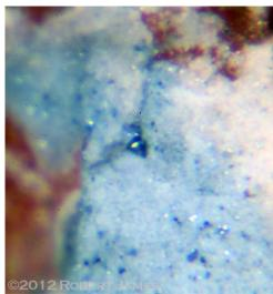
The black powder substance had a consistency that ran from quite fragile to very hard. The metal grains are ubiquitous throughout the surface of the specimens with concentrations in the grey powder material as seen at left in this image of an Abduriyim/Hughes specimen at 120x.
