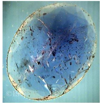
Based on our research methods and techniques used to expose the Tibet andesine fraud, we also were able to identify tubes of color infusion material in several of the rough tanzanite crystals we obtained, an example from that research is below.
