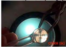
The 28 tourmalines all showed remarkably clear uniaxial interference figures in the polariscope, and all dead on center to the table of the stone.
